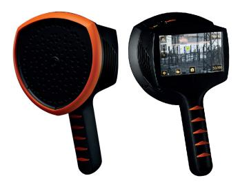
The NL Camera is an easy-to-use, stand-alone device for detecting partial discharge problems in high voltage electrical systems. The NL Camera utilizes 124 microphones to find sounds emitted by partial discharges – even when they are completely inaudible to the human ear. The located partial discharges are instantly superimposed on the camera view allowing the user to pinpoint and report possible problems visually.
