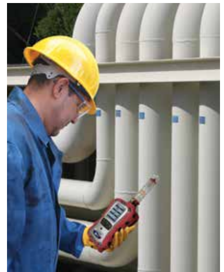
MultiRAE Benzene used for leak detection
