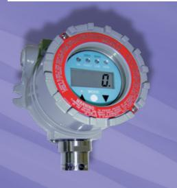
The RAEGuard EC is a permanently mounted (fixed) toxic gas or oxygen sensor/transmitter that operates from a 9 to 36 VDC power source and provides an analog (4 to 20mA) and digital (RS-485) signal output. Housed in an explosion-proof enclosure, the RAEGuard EC is equipped with a local digital display of the gas concentration and function keys for performing calibration. The RAEGuard EC is operated with a standard 4 to 20mA/RS-485 controller or as a stand-alone sensor module.
